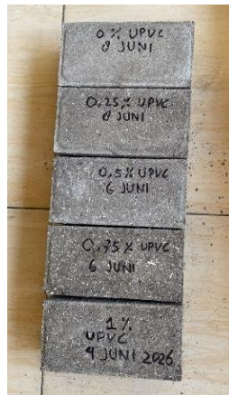
Gambar 2. Paving Block + UPVC
