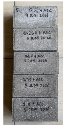
Gambar 3. Paving Block + UPVC + 2% Akselerator
