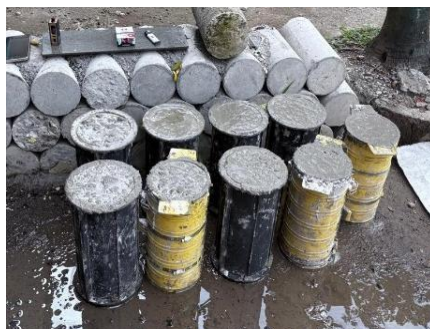
Gambar 3. Beton silinder ukuran 15 mm x 30 mm
