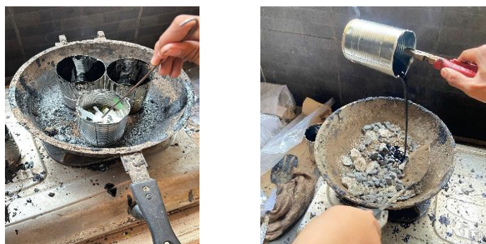
(a) Process Of Mixing Liquid Asphalt With LPDE Plastic (b) Asphalt Mixing Process With Aggregate
