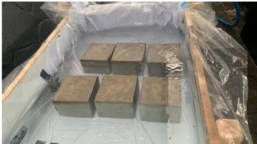
Gambar 4. Proses curing beton
