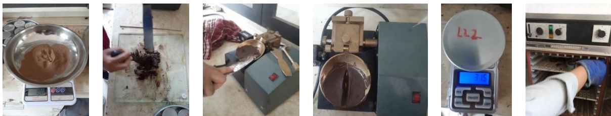
Gambar 10. Proses uji liquid limit
