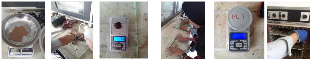
Gambar 12. Proses uji plastic limit
